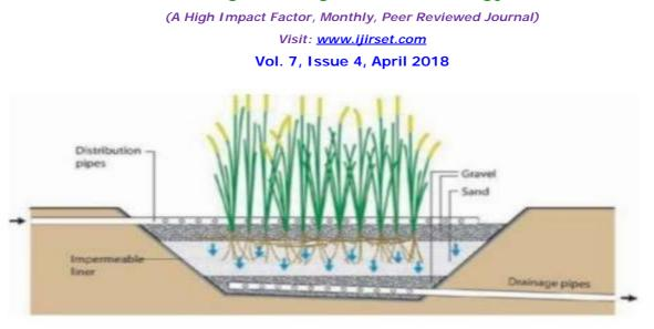
Figure -1 Schematic cross-section of vertical flow constructed wetland
